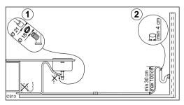
The waste connection must be at a height of between 30 cm (minimum) and 100 cm (maximum) from the floor.
